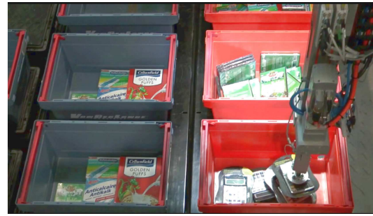
(b) Vanderlande gripper; flexible vacuum gripper, Vanderlande Industries BV (source: http://www.youtube.com/watch?v=4hjmLYvy5DI ). Product items are picked from product tote (red box), singulation, and placed into order tote (blue box), composing.
