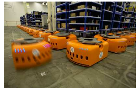
Figure 2.4: Kiva Mobile Fulfillment material handling system from Kiva Systems ( www.kivasystems.com ).
