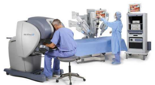
(b) Professional service: robot assisted surgery (Intuitive Surgical, da Vinci ® Surgical System)
